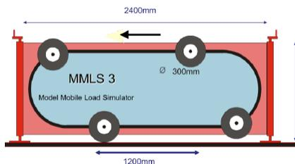
Schematic of the Model Mobile Load Simulator (MMLS3)
