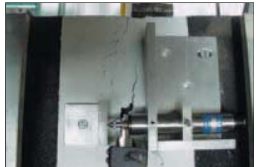
HaTelit® -reinforced sample: shearing after 570,000 cycles
