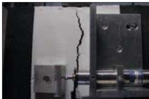
Unreinforced sample: bending after 80,000 cycles
