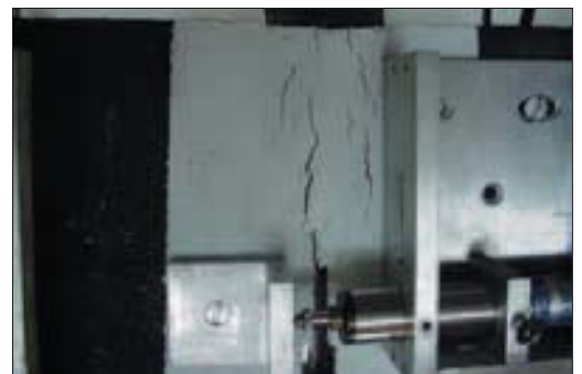
HaTelit® -reinforced sample: bending after 490,000 cycles
